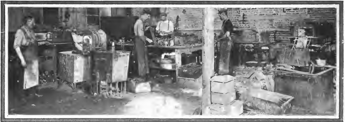
Fig. 12—Portion of heat treating department, with furnaces, quenching baths, and other facilities in actual service
